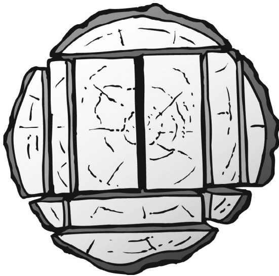
Figure 2. One way of sawing boards out of a log. The number of board feet of lumber that can be sawn from a log depends largely upon the sizes of the boards cut (Photo by T. E. Avery, from Avery, T. E., and H. E. Burkhardt. Forest Measurements , 3rd edition. McGraw-Hill Publishing Co., New York, NY. Reproduced with permission).
