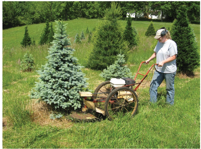
Figure 4. A motorized mower, as shown, is an asset to any Christmas tree operation. It can aid control of vegetation in and around the growing trees, and it can be used by the grower to clear alleys and walkways so as to maintain easy access to all areas of the production site.
