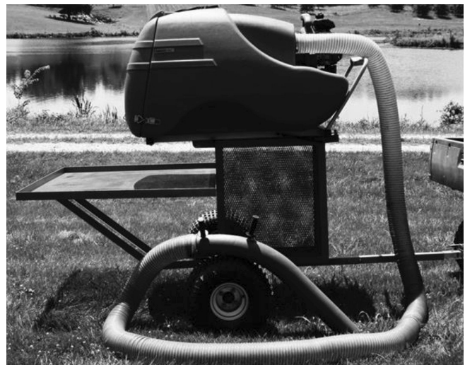
Figure 5. Greystone Vacuum's Maxi Vac on a raised trailer. (Used with permission from Warmund (2012, fig. 1 B).
