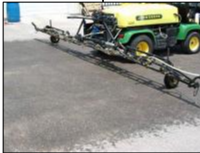
Figure 19. Check spray pattern uniformity by driving over a hot pad of road surface and watching the drying pattern.
