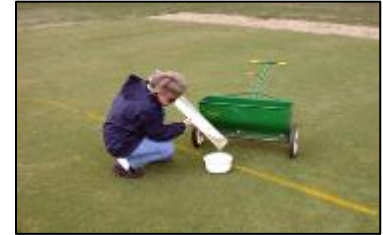
Figure 25. Attach a calibration pan beneath the spreader so that when the spreader is pushed over the calibration course, the output is collected.
