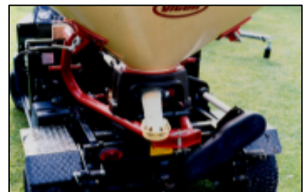
Figure 12. Centrifugal spreader powered by a tractor pto.
