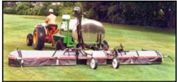
Figure 11. Shield booms minimize the effect of wind on the spray pattern and thereby reducing drift potential. control drift while still providing flexibility when you can spray, shielded booms have become increasingly popular. The shields fit over the boom
