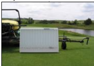
Figure 16. Check spray pattern uniformity.
