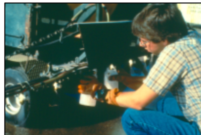
Figure 21. Nozzle output determination with calibrated containers and stopwatch.
