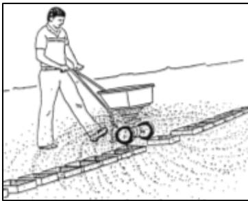
Figure 24. To make a quick check, lay out a row of shallow cardboard boxes at right angle to the direction of travel.
