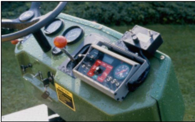
Figure 9. The control console and microprocessor for a spray controller.
