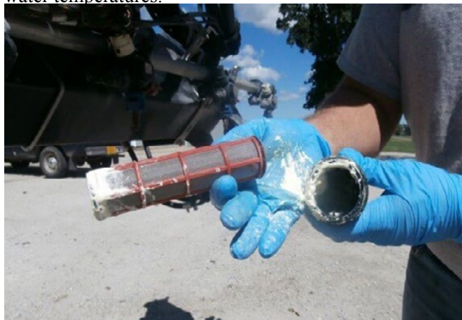
Figure 3. When certain pesticides do not dissolve in cold water, it can result in clogged filters. (Used with permission from Fred Whitford, Purdue University.)
