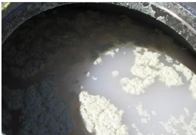
Figure 2. Clumping as a result of over-agitation in the spray tank. (Used by permission from Fred Whitford, Purdue University.)
