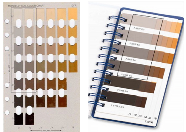
Figure 6. Left: An X-Rite soil color book (X-Rite, Grand Rapids, MI). Gray colors are inside the blackbox on any page. Gray is defined as having value 4 or more and chroma 2 or less on any page in the book. Right: The Globe Professional® book (Visual Color Systems, Kingston, NY). Gray colors are inside the black box on any pages with chroma 1 or 2.
