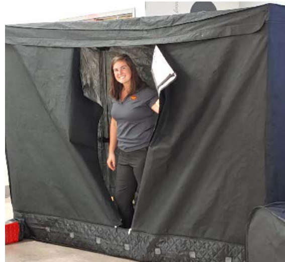
Figure 4. Heat Chambers can be kept on site to treat bed bug infested furniture. (Morgan Wilson, Virginia Tech)
