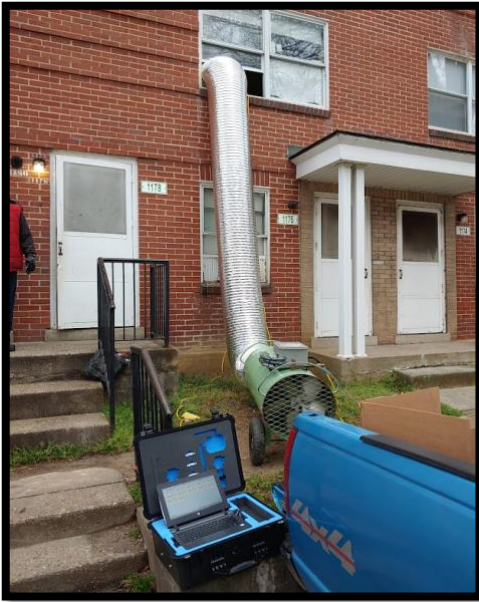
Figure 5. Researchers were monitoring indoor temperatures during a GreenTech propane heat treatment (Dini Miller Virginia Cooperative Extension)
