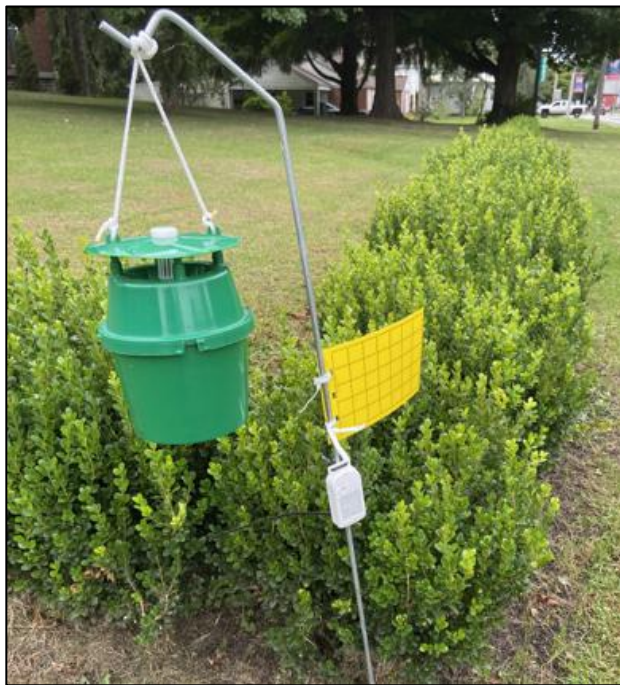
Figure 1. Adult bucket trap next to yellow sticky card and weather data logger. Photo by Alejandro Del-Pozo, Virginia Tech.
