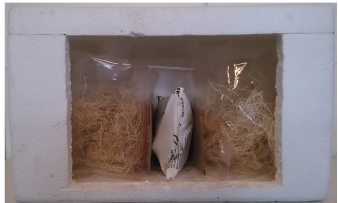
Figure 2. Cutaway showing two small, inflated bags in a cooler with a gel pack. This shipping method is good for smaller batches and has a high survival potential, but it is a suboptimal use of space.
