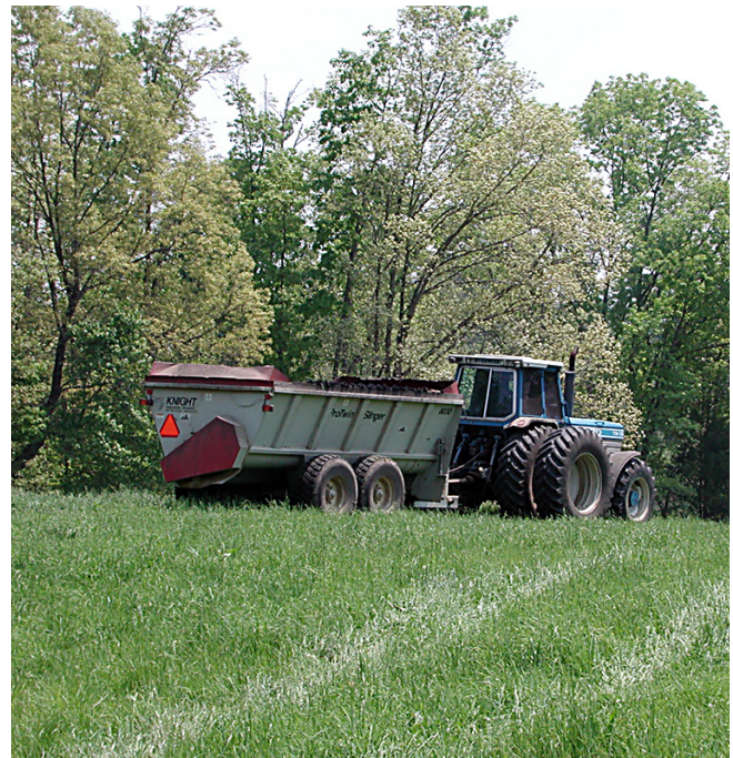
Figure 1. Tractor-drawn manure spreader applying biosolids onto a Virginia pasture in early May.
