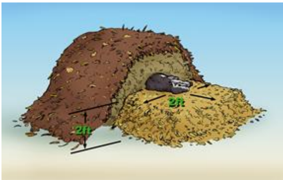
Figure 1: Composting Pile Construction Drawings by Bill Davis, Courtesy of Cornell Waste Management Institute
