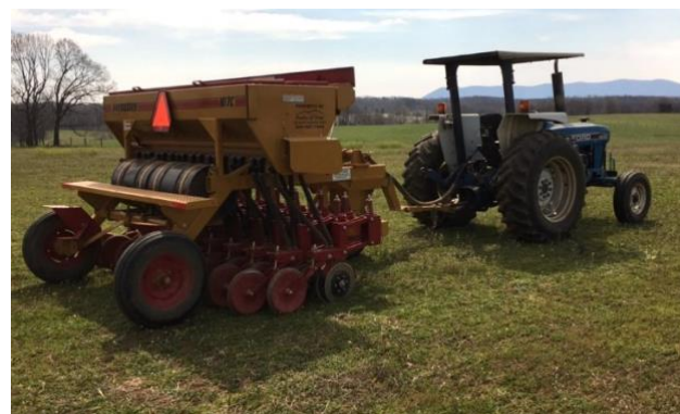
Figure 2. Keith Tuck planted his switchgrass using a Haybuster 107 C no-till drill rented from his local Soil and Water Conservation District (Photo. Keith Tuck).
